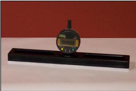
RWG-DF Digital Flat Roller Wave Gauges feature a flat, Delrin-coated bottom surface that is 16 inches long. The RWG-DF comes with a digital indicator for easy read-out of peak and valley measurements ( $W$ ). The gauge is used with a measuring tape to determine the roller wave length ( $L$ ), or the distance between two consecutive peaks or troughs (see diagram on next page). The digital gauge can be set to either inches or metric readouts and has a sensitivity of 0.01mm (0.0005 inches).
