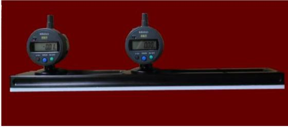
This dual-gauge model has a 16-inch (406 mm) base and is specifically designed for measuring edge-lift (edge curl) in heat-treated flat glass (a requirement of EN 1863-2 and EN12150-2), but can also be used as a flat-bottom roll-wave gauge. Ideal for production control & incoming QC. Controlling edge-lift reduces optical distortion and the chance of field failures in laminated units.
