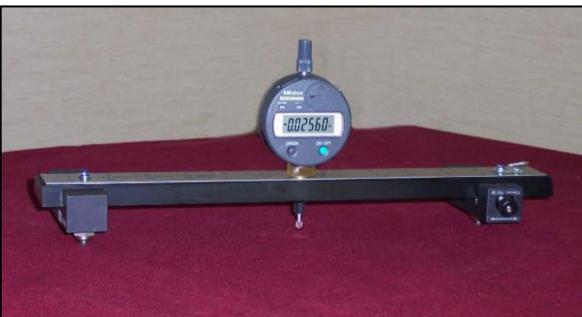
The RWG-D Digital Roller-Wave Gauge features a non-wearing, three-point contact bottom surface and digital indicator readout with a metric resolution of 0.01 mm or an inch resolution of 0.0005 in. The contact point spacing is adjustable to the length of the peak-to-peak roller wave distance for more accurate, repeatable results. A high-sensitivity model (RWG-D-HS) is available for applications requiring high distortion sensitivity (1 mdpt).
