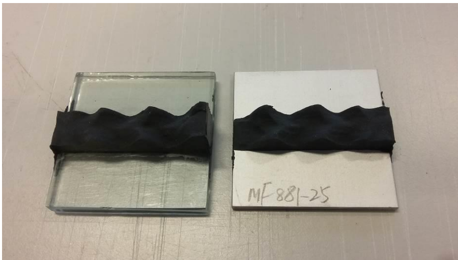
Sample type 1 (H-sample) typical failure pattern
