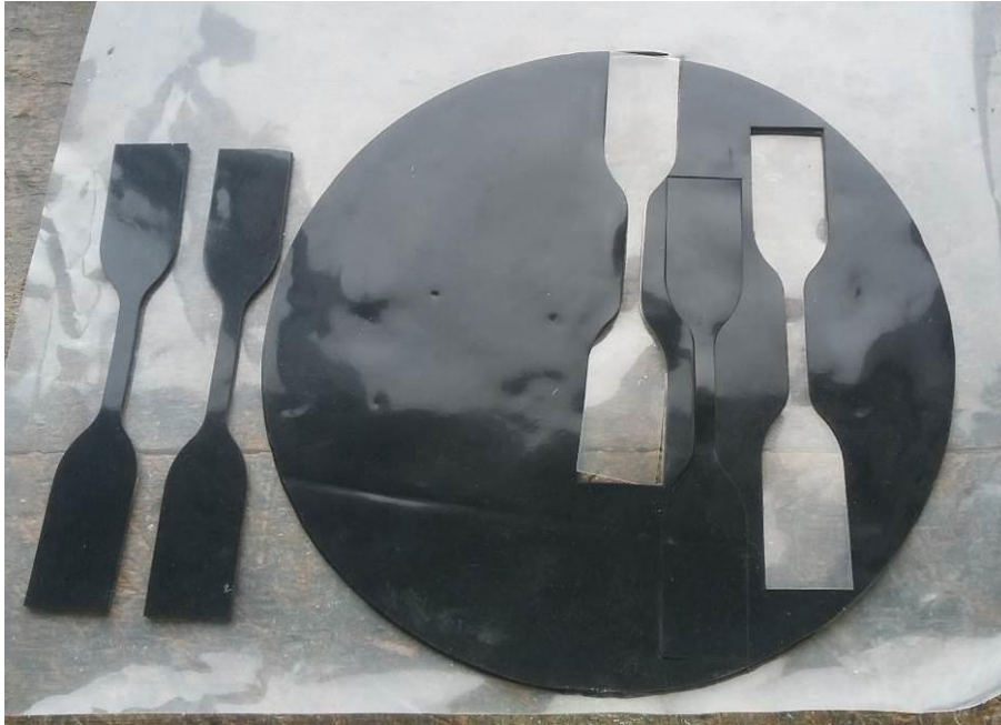
Sample type 2 and ISO 527 type 5 specimens punched from 2 mm sealant film
