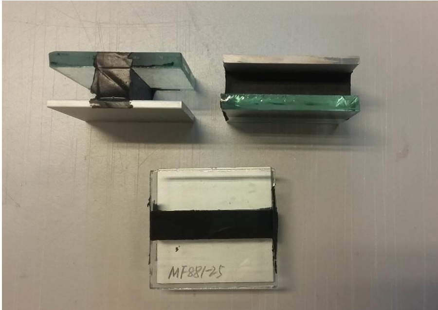
Sample type 1 (H-sample) 6 mm float glass. 3 mm anodised aluminium. seal joint 12x12x50 mm
