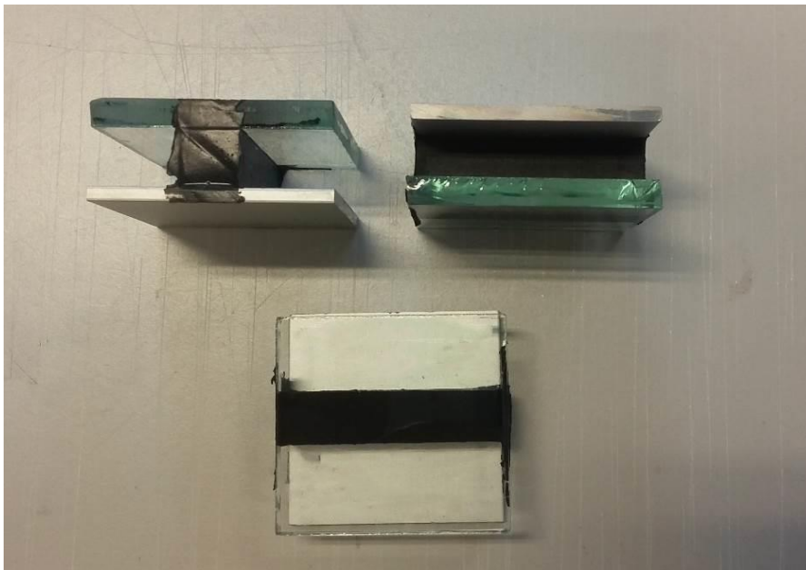
Sample type 1 (H-sample) typical failure pattern
