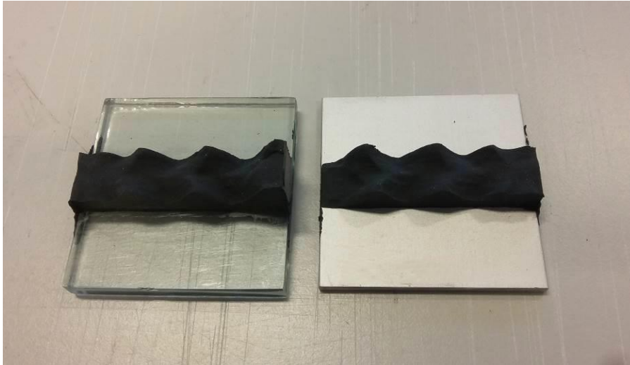
Sample type 1 (H-sample) 6 mm float glass. 3 mm anodised aluminium. seal joint 12x12x50 mm
