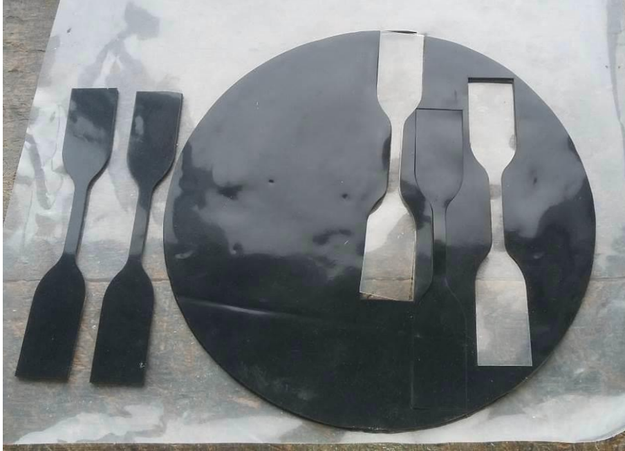
Sample type 2 and ISO 527 type 5 specimens punched from 2 mm sealant film
